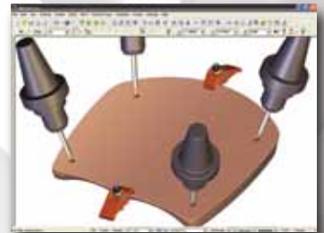
Specialized toolpaths support fast, efficient 5-axis drilling.
